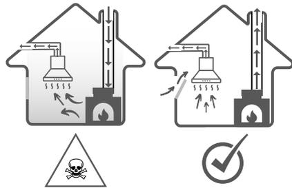
If there is not enough air supply, a negative pressure is formed. Toxic gases from the chimney or the exhaust pipe are recirculated in the rooms of the house.
