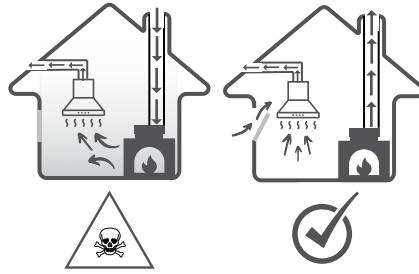
If there is not enough air supply, a negative pressure is formed. Toxic gases from the chimney or the exhaust pipe are recirculated in the rooms of the house.
