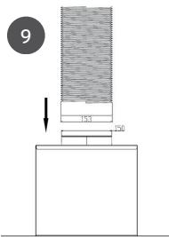
EN 5.10 Installation of the air adapter (reduction)
